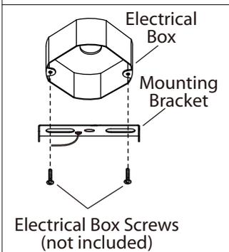
**2.** Mount the mounting bracket to electrical box using electrical box screws (not included).
