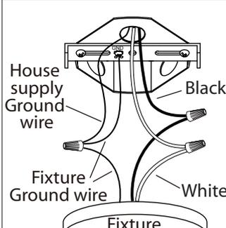
**3.** Connect the ground wires (bare copper or green) from your fixture to the ground wire (bare copper or green) or ground screw in the electrical box. Connect the black wire (or wire with marking) from the fixture to the black wire in the electrical box and connect the white wire from the fixture to the white wire in the electrical box.
