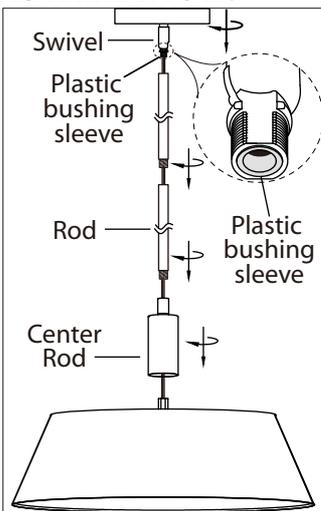
**1.** Screw the center rod to the fixture. Install the length of rod that is required by threading wire through the rod and screwing it to the fixture. Install swivel to the rod, ensuring that the plastic bushing sleeve is at the swivel.
