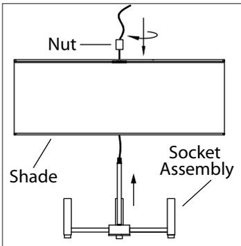
1. Install the socket assembly to the shade by tightening the nut.
