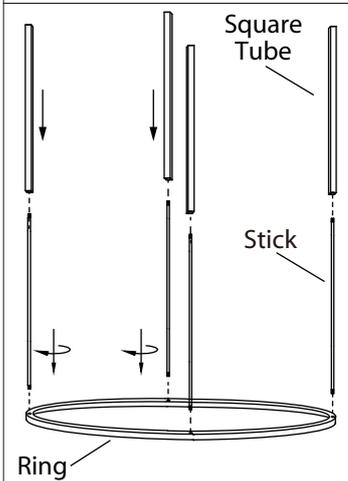
2. Remove the nuts from the sticks. Screw the 4 sticks onto the ring then insert the square tubes over the sticks.
