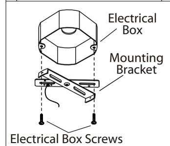
5. Mount the mounting bracket to electrical box using electrical box screws (not included).
