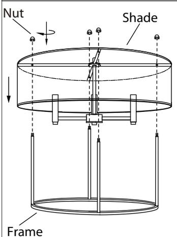
3. Install the frame to the shade by tightening the 4 nuts.
