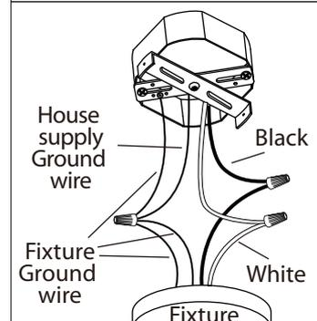
6. Connect the ground wires (bare copper or green) from your fixture to the ground wire (bare copper or green) or ground screw in the electrical box. Connect the black wire (or wire with marking) from the fixture to the black wire in the electrical box and connect the white wire from the fixture to the white wire in the electrical box.
