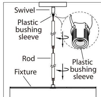
4. Install the length of rod that is required by threading wire through the rod and screwing it to the fixture. Install swivel to the rod, ensuring that the plastic bushing sleeve is at the swivel.
