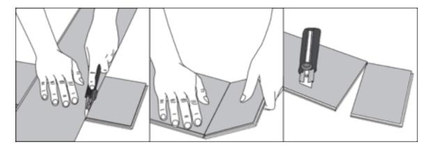
5. Start the second row with the leftover cut part of the last plank of the previous row. This small plank should measure at least 12". Otherwise, use another plank that should be cut in two. The end joints of each adoining row should not be closer than 8" to each other.
